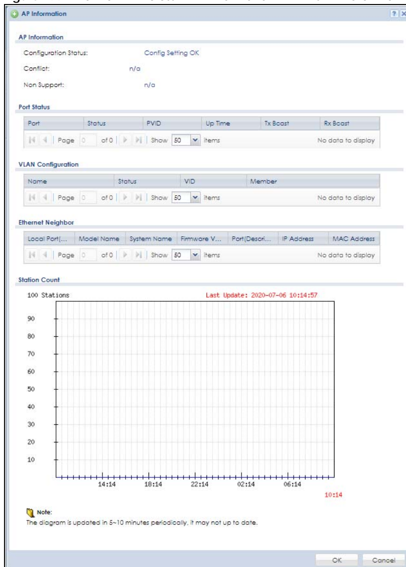
Figure 199 Monitor &gt; Wireless &gt; AP Information &gt; AP List &gt; More Information
